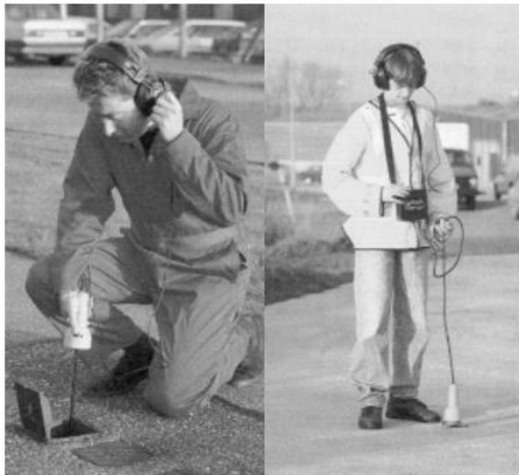
Gambar 2.9 Cara kerja ground microphone
