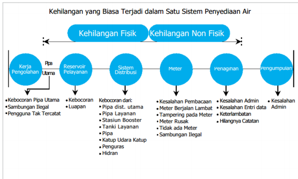
Gambar 2.5 Faktor penyebab kehilangan air (Sumber :The Manager’s Non-Revenue Water Hanbook: A Guide to Understanding Water Losses, 2008)
