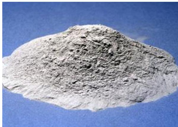
Gambar 2.3 *Fly Ash* (Sumber : Data Sekunder, 2017)
