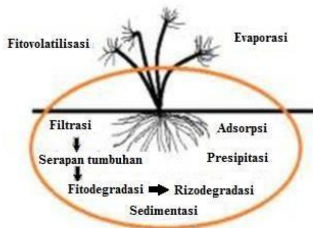
Gambar 2.1 Mekanisme Constructed Wetland (Khapre, 2015)
