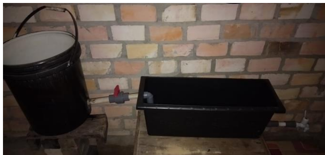
Gambar.7 Gambar Alat Surface Flow Wetland
