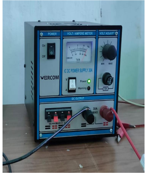
Power Supply DC
