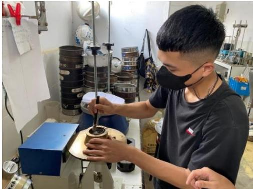
Proses Penumbukkan Flow Test
