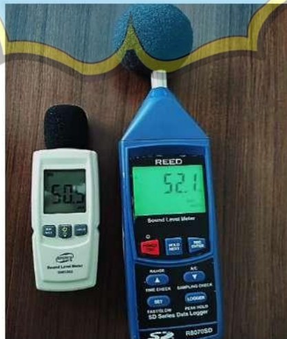
Gambar 4.12 Kalibrasi Alat Sound Level Meter
