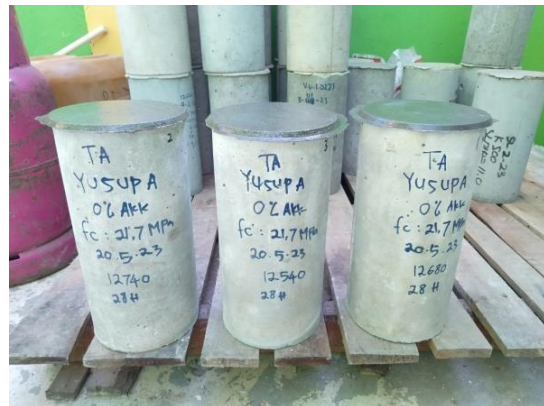
Capping benda uji
