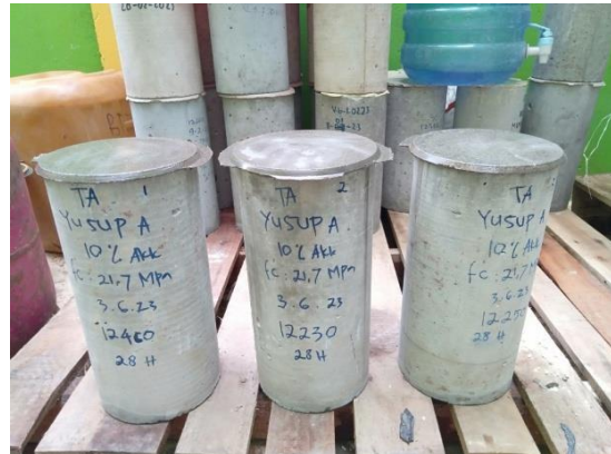
Capping benda uji
