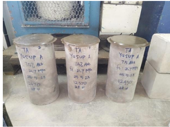
Capping benda uji
