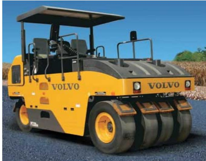
**Gambar 2.3 *Pneumatic tyred roller***
