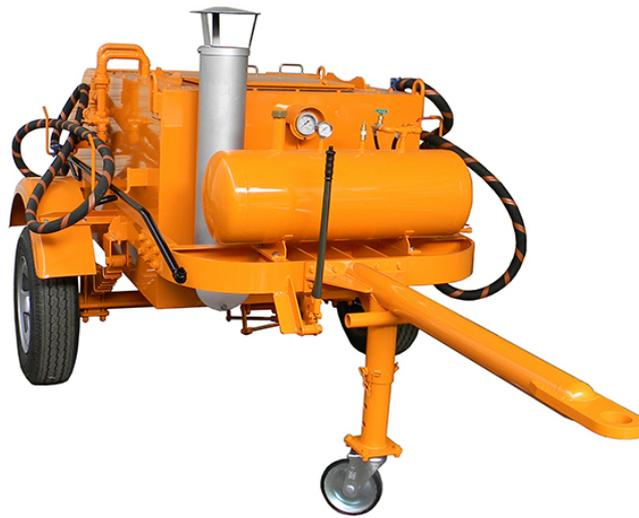
**Gambar 2.4 Asphalt Sprayer**
