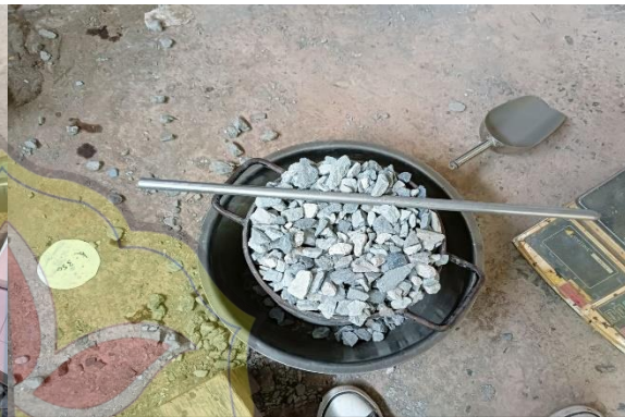
Gambar 2. Proses Perataan Agregat Kasar
