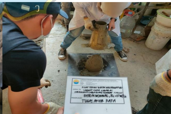
Proses Pengujian Slump
