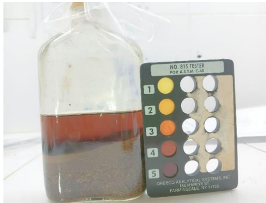
Gambar 4.2 Hasil Uji Kotoran Organik Pasir Dicuci Air (Standar Warna No.3)
