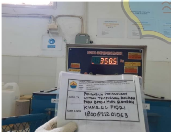
Nilai hasil uji kuat tekan beton silinder No.
