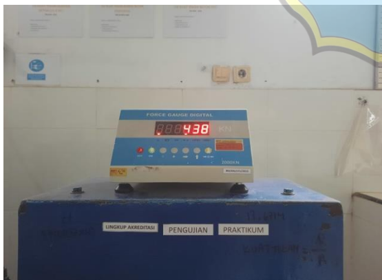
Nilai hasil uji kuat tekan beton silinder No.
